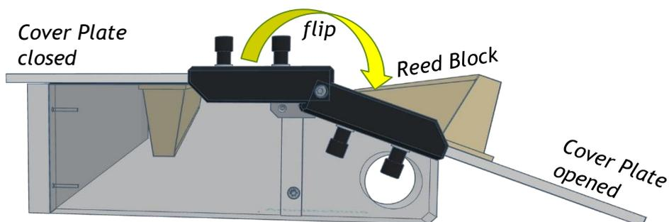
high frame with a sealed top plate, which has an audible effect on the measured pitch and sound. In addition, a cassotto can be activated, which simulates e.g. the space on the bass side between the filling and the finger plate, or the treble cassotto on an accordion.
