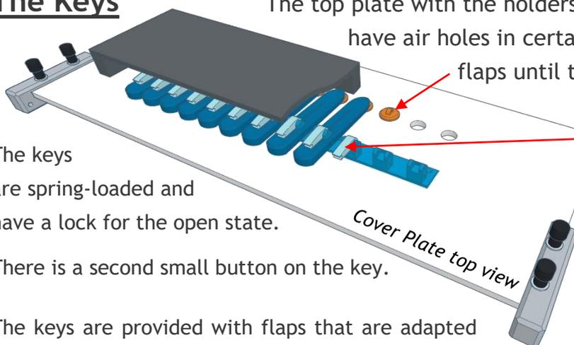
Round, oblong or triangular keys are possible. Custom key shapes are also possible. For single reed plates and reed blocks the air vents have a diameter between 10 and 14 mm, for helicone basses 30 mm.
