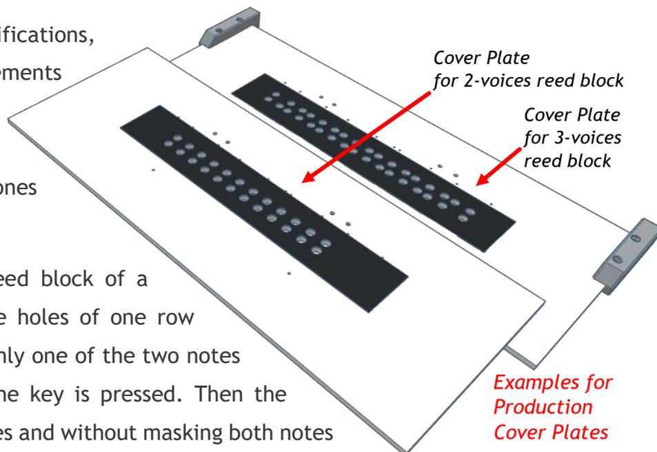
Due to the simple and quick exchange of the cover plate, it is possible to change from one hole pattern to another. The cover plate always includes all keys and optionally a cassotto. Parts of the reed block holder can be used on the next one when changing the cover plate. The length of the reed blocks can vary between 15 cm and 42 cm.
