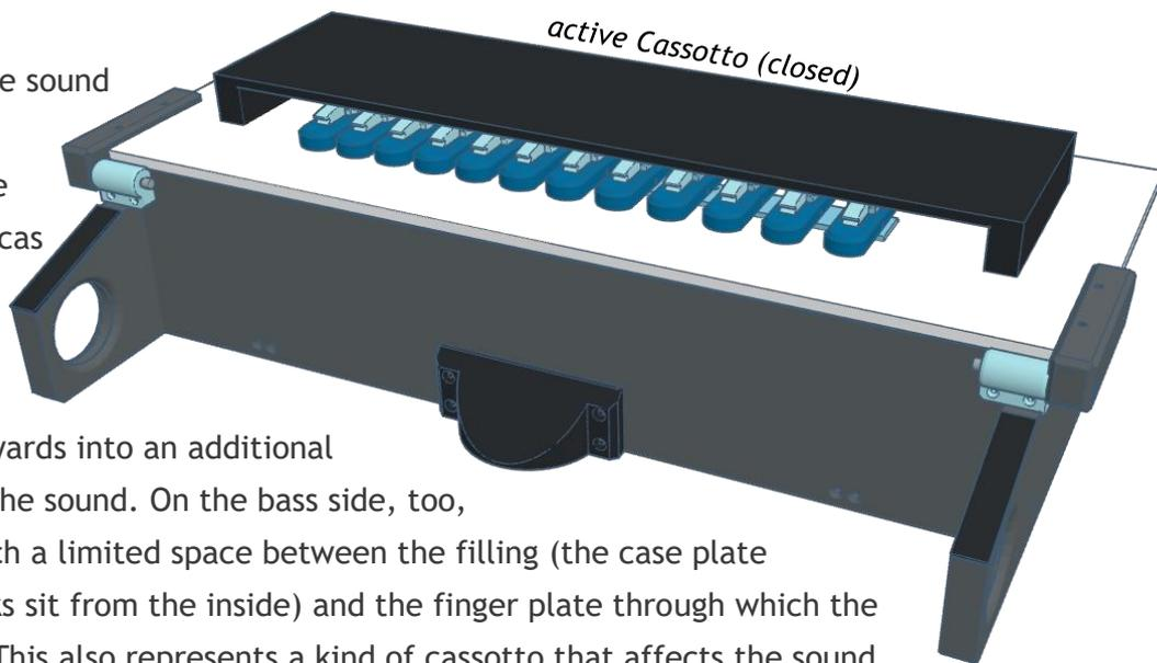
**AKKOflip** is equipped with a cassotto as standard. This consists of a hood that is attached to the rear part of the top plate with two hinges and can be folded forward. When closed, the hood is held closed magnetically and forms the additional resonance volume of a cassotto. By folding it open and closed, a comparison of the sound without and with the cassotto is possible.
